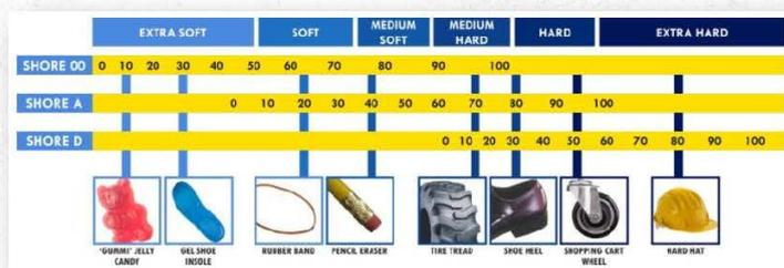
The **Shore A** Hardness Scale measures the hardness of flexible mold rubbers that range in hardness from very soft and flexible, to medium and somewhat flexible, to hard with almost no flexibility at all. Semi-rigid plastics can also be measured on the high end of the Shore A Scale.
