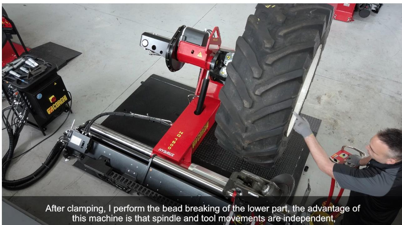
After clamping, I perform the bead breaking of the lower part, the advantage of this machine is that spindle and tool movements are independent,
