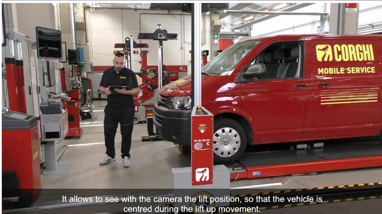
It allows to see with the camera the lift position, so that the vehicle is centred during the lift up movement.
